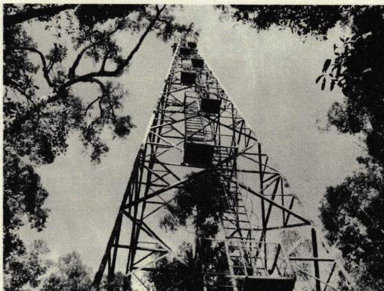
40-m-tall tower for CO 2 and energy flux measurement in an Indonesian peat swamp forest (T. Hirano)
